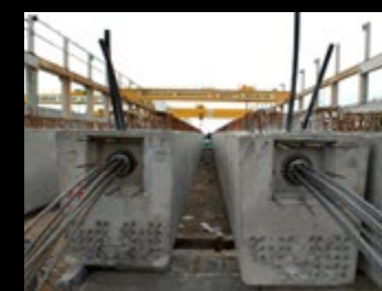
Trapeze beams, post stressed
